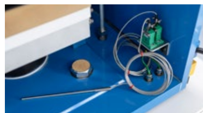
Connection for external thermocouple
