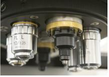
the test to be performed. The turret can be configured with one or two indenter actuators, and combined with a maximum of four objectives. The second indenter can be added after installation.
