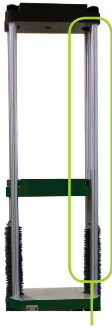
On this 150SL frame the columns have been extended to accommodate large test specimens.
