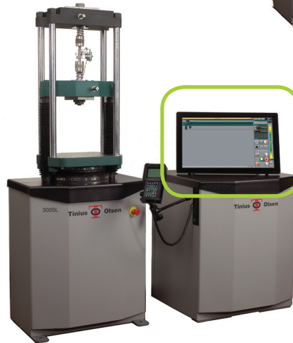
Typical 300kN (60,000lbf) SL with optional computer running Tinius Olsen's Horizon software.
