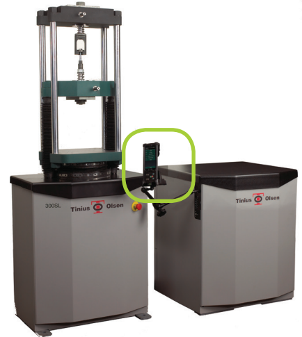
Typical 150kN (30,000lbf) SL with handheld controller.
