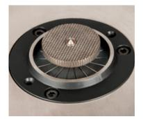
Lower radial v-groove die with large, serrated rotor. The low-mass rotor design ensures homogenous temperature distribution, and in conjunction with MonTech longlife seals, offers the highest accuracy in Mooney readings.
