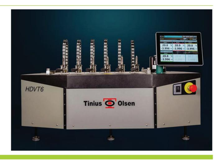
HDT - Heat Deflection (or, distortion) Temperature DTUL - Deflection Temperature Under Load Vicat Softening Temperature
