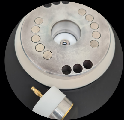
setup with 10 circular permanent magnets in the base of the LUXOR coater
