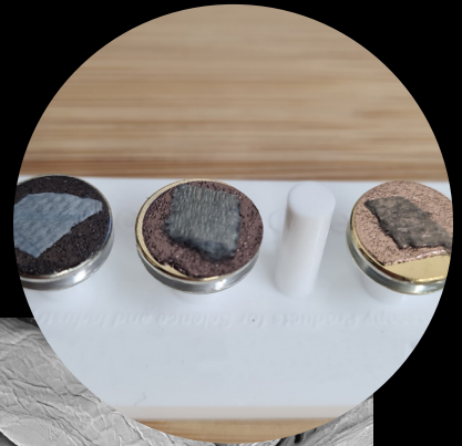
from left to right 2 nm, 5 nm and 10 nm gold coated paper tissue samples on aluminium stubs
