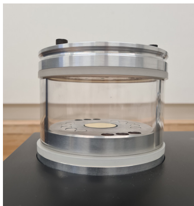
the simple setup of the coating reactor
