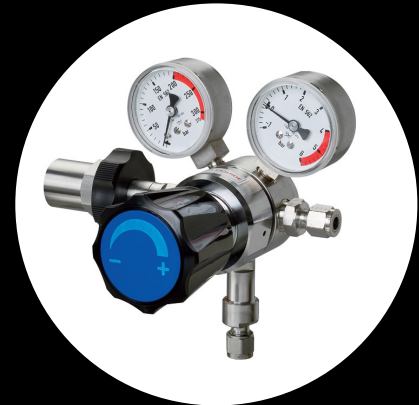
pressure regulator with 2 pressure dial gauges. The left gauge shows the pressure in the gas cylinder, while the right gauge allows for a fine adjustment towards the sputter coater
