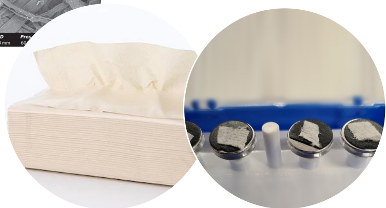
tissue paper samples on 12 mm aluminium sample holders fixed with double sided carbon tape
