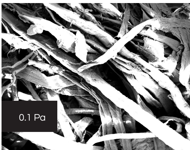
SEM imaging of tissue paper at 60, 10 and 0.1 Pa. Magnification 1.000x, 10 kV, BS detector
