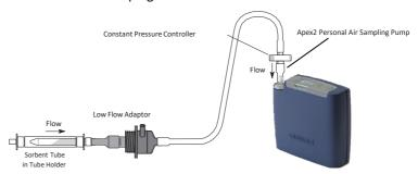
Above is a typical sample train using a sorbent tube. The ends of the sorbent tube are broken off and inserted into a tube holder which is then connected to a personal sampling pump. Generally the flow is lower (typically 20-200ml/min) and so either a dedicated low flow pump may be used or a medium flow pump, e.g. a Casella Apex2 with a Low Flow Adaptor. The flow rate needs to be set and checked pre and post sampling.
