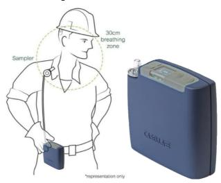
A personal sampling pump would be connected to a sampling head containing a suitable filter via a length of tubing. The pump is normally worn on the belt, but it can be mounted on the back or the chest in a suitable harness. The sampling head, however, must be in the breathing zone for a valid sample.
