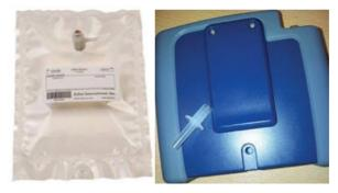
Attach the Tedlar bag to the outlet of the pump using a suitable length of tubing and a luer fitting e.g. Casella TUC12. In some pumps, the bag fill mode is automatic. Once the pump is set running, the pump will stop automatically when it senses the bag is full. If your pump does not have this feature, work out the time you need to fill the bag. Take care not to overfill the bag.
