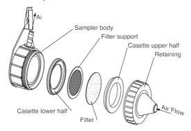
Like the IOM-type head, the CIS head has the advantage of being able to sample different size fractions simultaneously through the use of PUF filters. See PUF Filters for Size Selection for description of its use with PUF filters.
