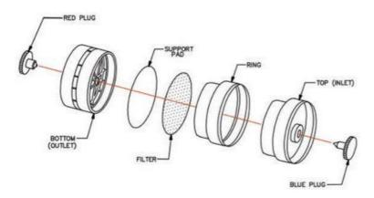
Please take care to attach your cassette the correct way. The wagon wheel design at the base is the outlet face, otherwise your sample will be deposited on the support pad.
