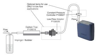
Above is a typical sampling train for an impinger. An impinger may be mounted on the side of an air sampling pump or put into a special holster and placed need the worker's breathing zone.
