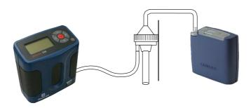
The MESA Defender is an example of a Primary Calibrator and works by detecting and timing a passing piston electronically. The flow rate is displayed on the LCD screen. Mass flow type primary calibrators are also available in the market and are equally as simple to use.
