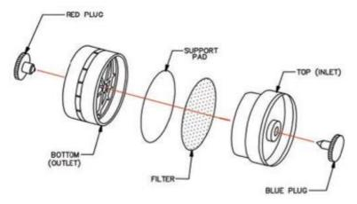
Closed face sampling refers to sampling where only the plugs are removed, and air is drawn through the filter. A 2-piece cassette is better for this because the cassette itself exerts electrostatic forces which attract the contaminants to the walls of the cassette and a 2-piece cassette has less surface area for contaminants to cling to instead of being caught on the filter.
